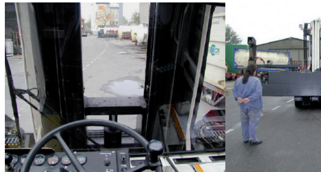
Front view obstructed by window pillar; the driver is not in a position to see his companions.
