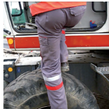
Operator descending instinctively using the tires instead of the unergonomic access system.
