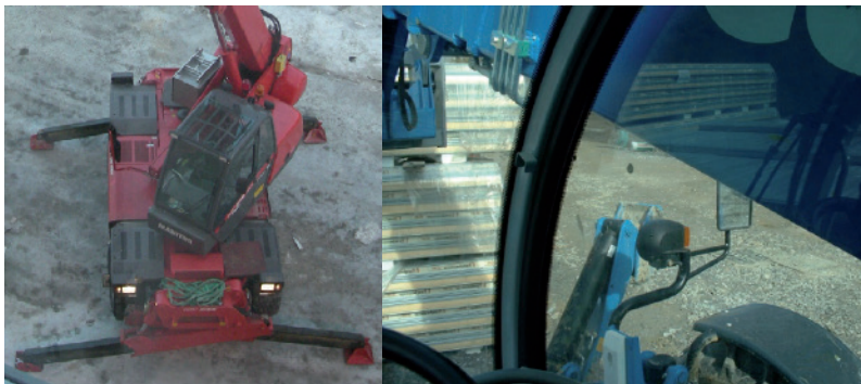
Machines with side boom; side view obstructed by the boom.
